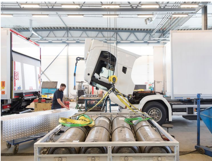
Hydrogen tanks inside the Scania regional service center of Trondheim. Photographer: Rocco Rorandelli for Bloomberg Businessweek
